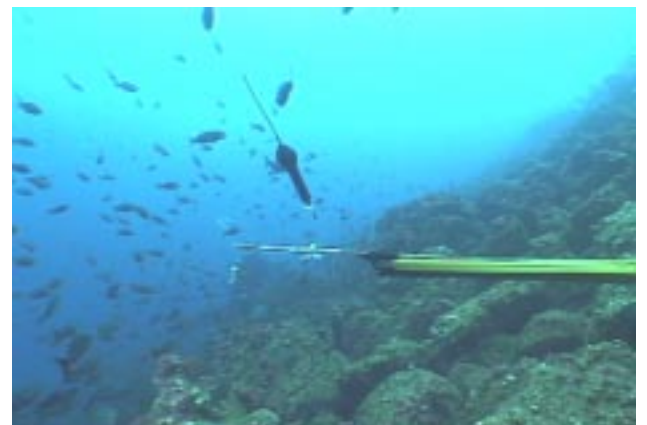
The small size and minimal drag coefficient of the new pop-up archival tags permits them to remain attached to the host animal for much longer time periods.
